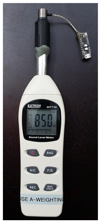
sound meter. Oil-based clay or other suitable putty material is used to seal the coupler to the ½ inch microphone stem of the digital sound level meter. Note that the coupler may be a 3D printed component and attached to the digital sound meter as shown in the figure above.
