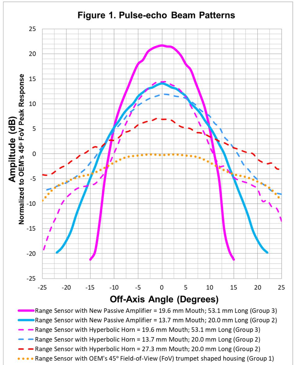
sensor operating at ~80 kHz (~4 mm wavelength). This specific MEMS ultrasonic range sensor limits range detection to 5 meters in hardware.
