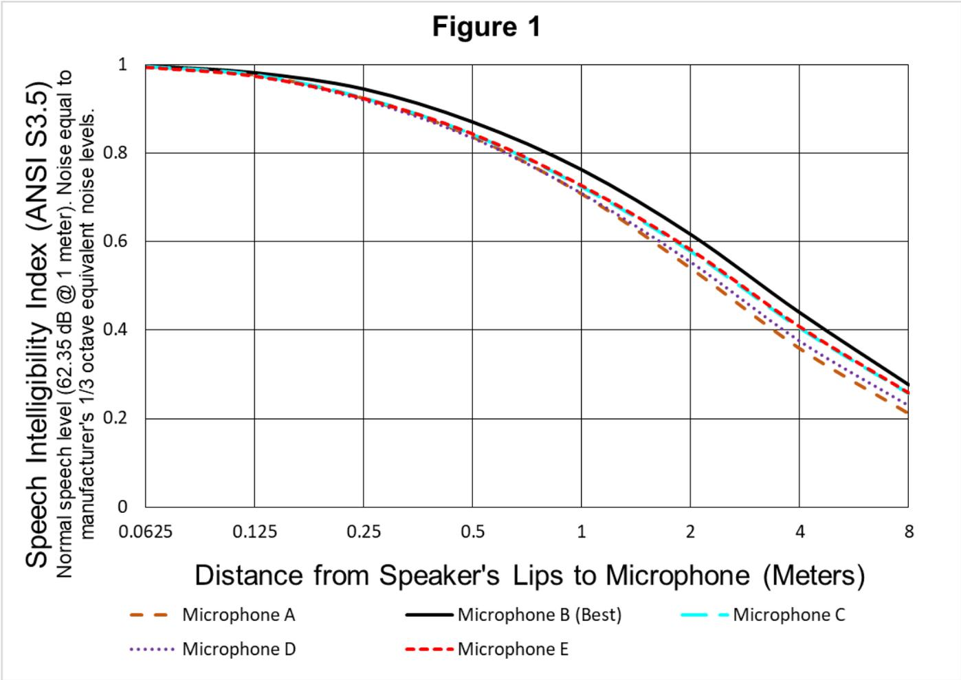
Figure 1 shows the maximum theoretical SII using this best-case model for five different, common, small microphones using the microphone manufacturer's published 1/3-octave equivalent noise levels as the only noise sources.
