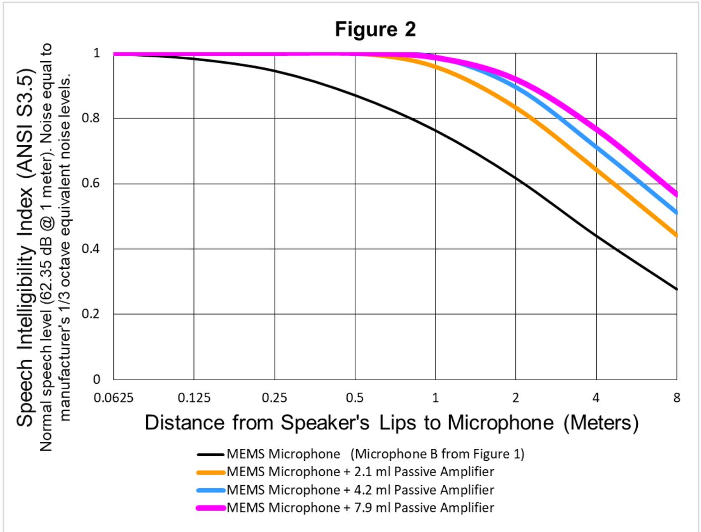
window, hardwood floor) so as to be more representative of difficult, real-world, listening conditions. White noise recordings were used to suppress standing waves which might corrupt audio measurements. The white noise used had balanced power spectral density. The white noise was attenuated 48 dB per octave at band limits. Both the speaker and the microphone were free-standing on 16 mm poles, 1.4 meters above the floor and separated by 1 meter.
